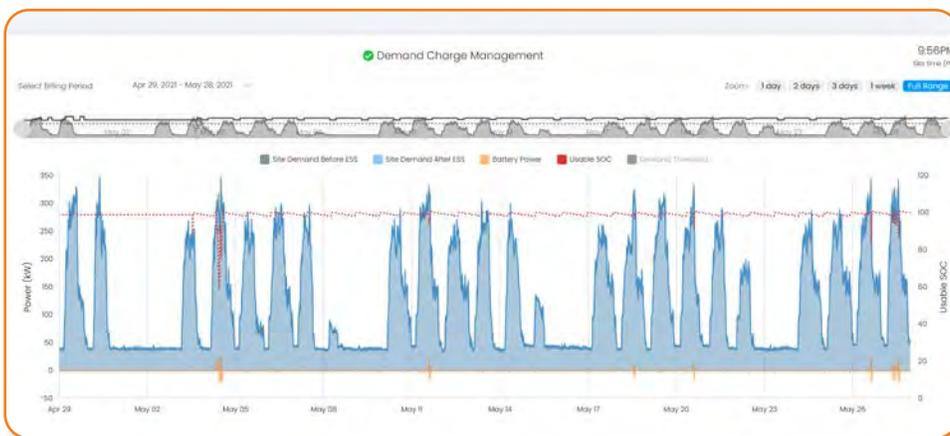
The monthly data (left) for the American Faucet factory are punctuated by relatively narrow and extreme peaks. While the ESS capacity is just 7.6% of the peak load, Acumen EMS is highly successful at dispatching stored energy to offset NC demand. The daily data (above) shows the maximum NC demand with and without ESS. On this key day, the 29.4 kW-rated battery shaved the midday peak demand by 28 kW.
